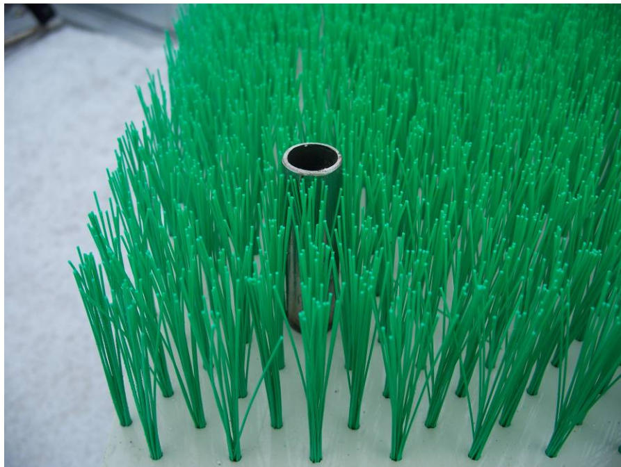
Figure 4.8: Bristle board with stainless steel spacer / nut
