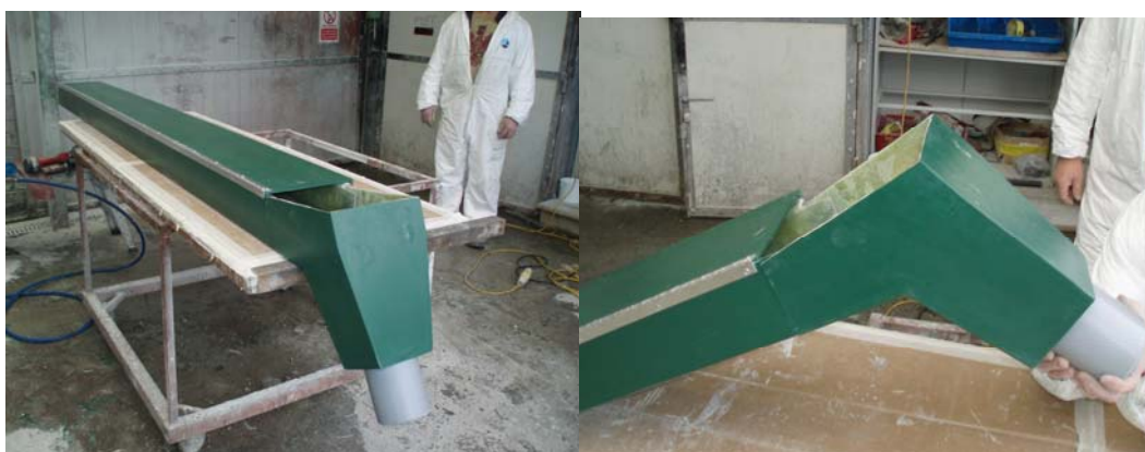
Channel with flow-splitter attached
